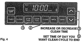
Note: When selecting a stop time for a delayed clean cycle, you must allow time for the 2-4 hour clean time.
